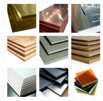
Aluminum Alloy 1100 is the most popular grade of aluminum for general purpose sheet metal works where moderate strength is the requirement. AA 1100 is also known for its excellent corrosion resistance, high ductility & reflective finish.
